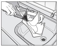
Clean the fabric conditioner channel using a brush and warm water.
